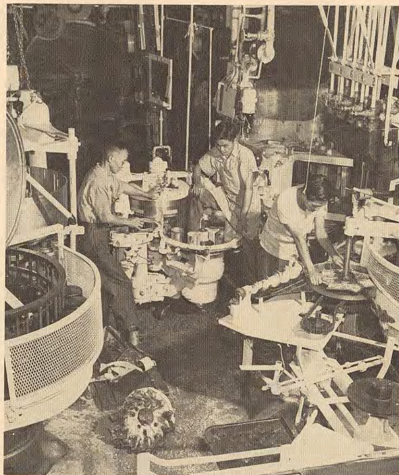
COMPLICATED MACHINERY Double seamer which must remain in top operation condition day and night during peak season is checked by K. Kono, left, K. Matsukado, center, and Clay Shinto.
